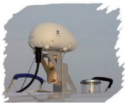
The Thorium™ : CLS' Iridium-based LRIT terminal
